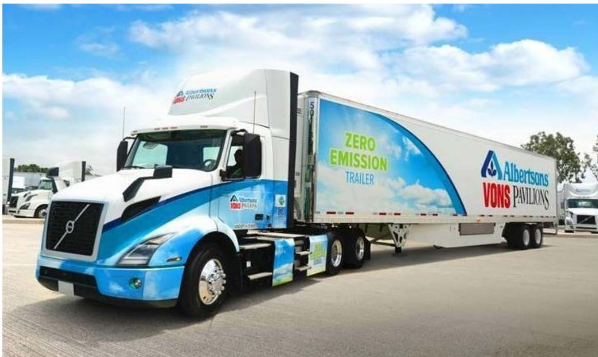
A Volvo VNR Electric paired with an electric-powered transport refrigeration unit from Advanced Energy Machines (AEM) made the first commercial 100% zero-emission grocery delivery with a Class 8 truck in the U.S. Volvo Trucks
